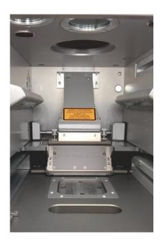
In addition, the SLM $^{\circ}$ 125 provides a **build volume reduction** of 50 x 50 x 50 mm $^{3}$  thus decreasing the amount of powder by 80%
