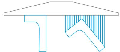
The part on the left is oriented directly against the build head and has a stable center of mass, so it doesn't require supports in this orientation. The part on the right is oriented such that it needs supports and has an unstable center of mass.
