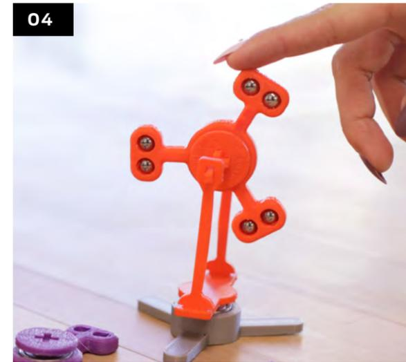
One partner will hold the rotor in place with one hand and apply a consistent rotational force on the fidget spinner each time. Immediately after spinning the fidget spinner in place, release the rotor being careful to avoid applying a sideways force.
