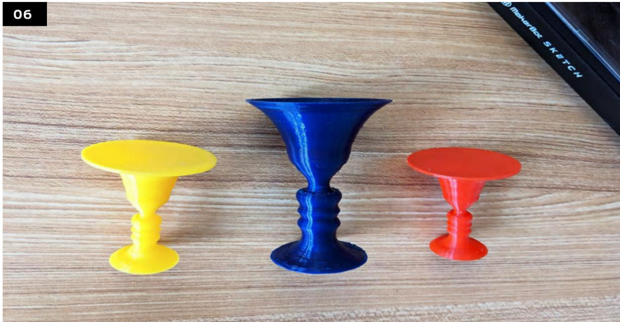
Prepare the file to print. We recommend orienting the model upside down to reduce print time and the need for printed supports.
