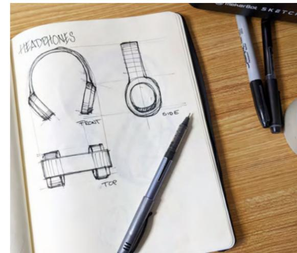
**Orthographic:** An orthographic sketch is a sketch drawn in one perspective. This means that an orthographic sketch can only communicate a fraction of a proposed idea. These sketches will typically be drawn either from a straight-on view, top view, front view or side view.
